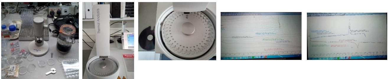
Differential scanning calorimetry (DSC) analyses of Pinus densiflora seeds. From left to right: sample preparation, measurement, and data outputs as thermal scans.
